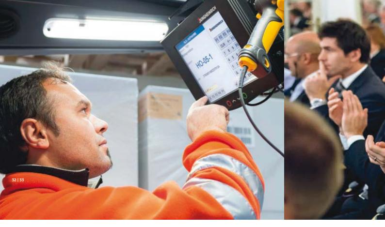
Optimized material flows: A Streng Plastic employee controls the Jungheinrich Warehouse Management System via a screen on the stacker.
